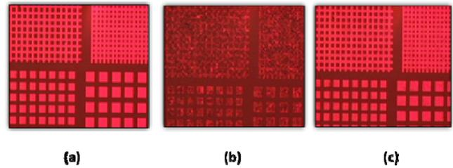
**Figure 6.** Copper patterns on test chip (a) after 30 seconds of formic acid vapor, (b) after a few seconds of atmospheric ambient, and (c) after formic acid flow is reinstated, showing the rapid reduction of the oxides.
