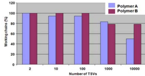
Figure 9. Electrical yield on 1000 TSV daisy chain structures with collective hybrid bonding method. Courtesy of Anne Jourdain of IMEC.
