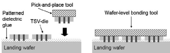
Figure 8. Illustration of Collective Hybrid Bonding, where accurate placement of TSV die is followed by gang bonding of all dice to complete the bonding process. Courtesy of Anne Jourdain of IMEC.
