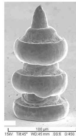
Fig.7 – Triple stud bump
