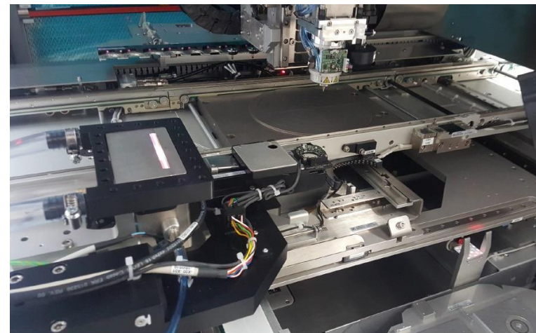
Example: BESi 2200 EVO With integrated Ontos Plasma Head for die activation
