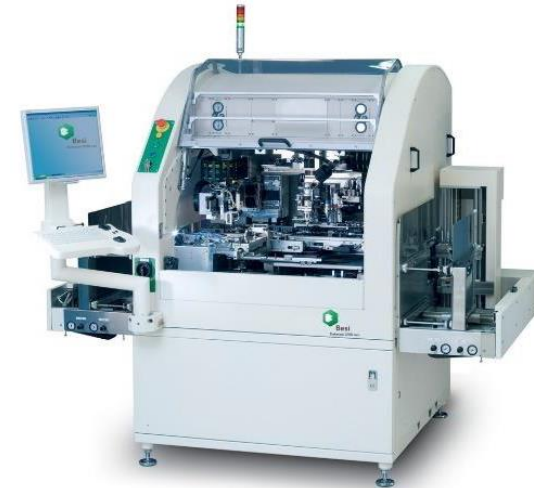
Example: BESi 2200 EVO With integrated Ontos Plasma Head for die activation
