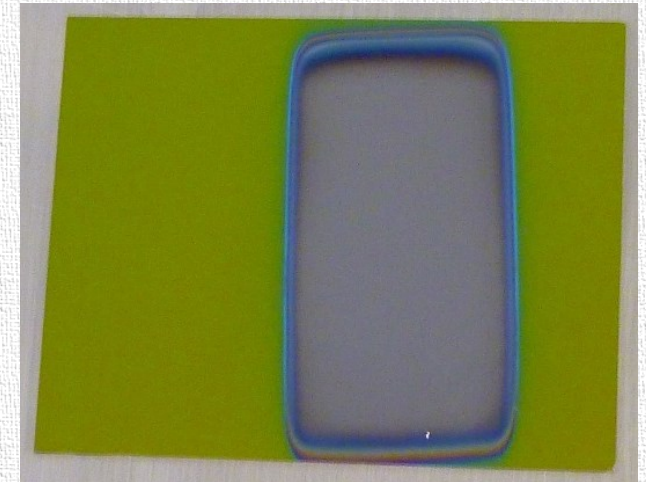
300 nm of i-line photoresist removed (RT, Ontos Oxidizing Chemistry)
