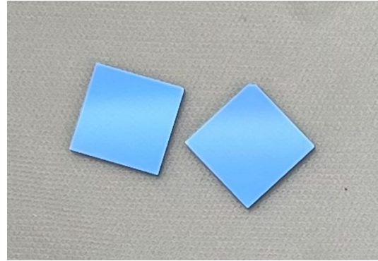
Untreated samples debonded with little force
