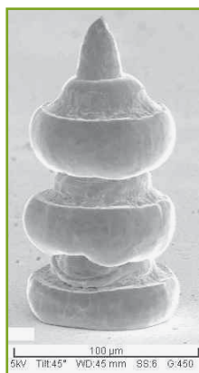
Figure 7: Triple stud bump.
