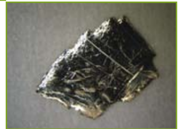
Figure 5 - Behavior of AuSn perform upon reflow.
