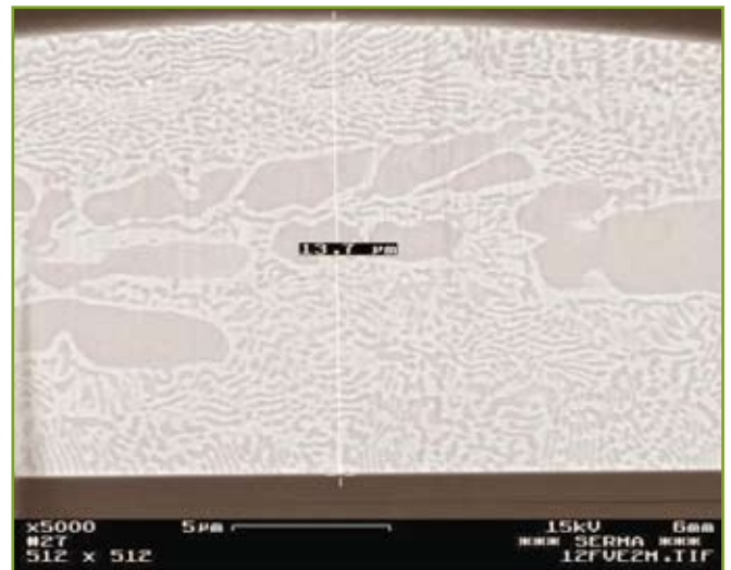
Figure 6 - SEM Image of a reflown sample showing the formation of the Au-Sn eutectic phase.
