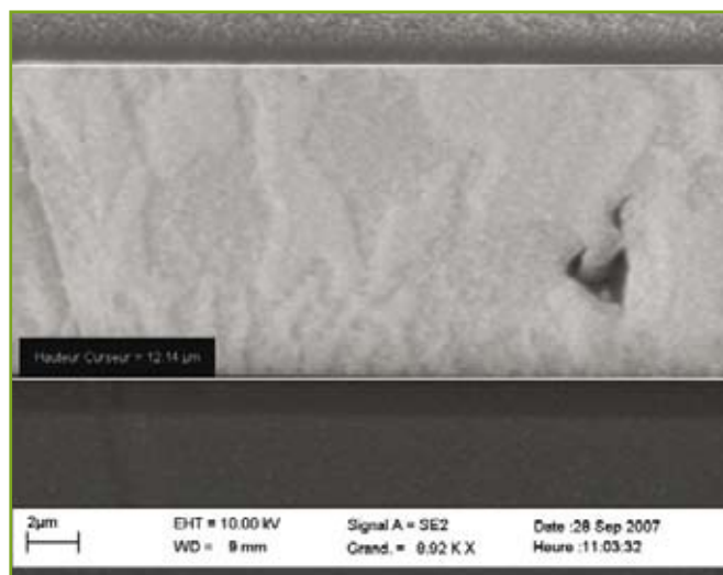
Figure 14 - Voids within the ring after reflow assembly.
