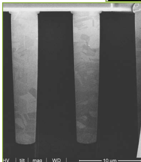
Figure 1 - Schematic of the 3D-SIC Through Silicon Via (TSV) module. Figure 2&3: FIB through TSV in vicinity of device after etch, strip & clean (left), and after TSV CMP and sintering (right). (Pt on top for contrast).
