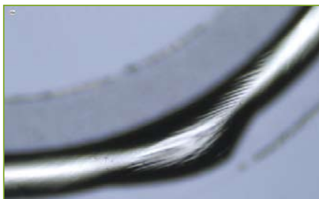
Figure 8 - Local material excess upon reflow.
