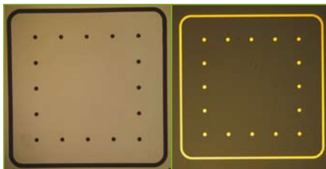
Figure 2 - Test samples: Seals rings and output pads on the silicon substrate and lid.
