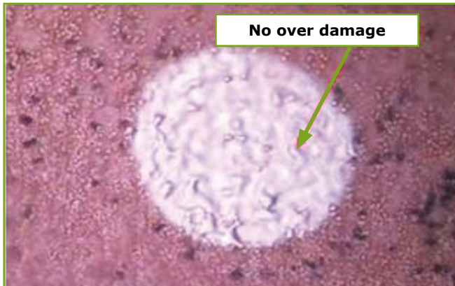
Figure 3 - Copper foil after removing 18μm carrier.
