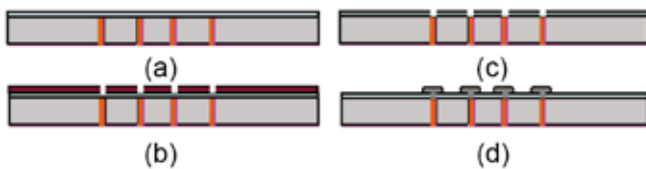
Figure 5 - Process flow for ENIG plating on top of TSV.
