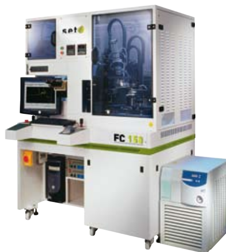
Figure 9 - SET FC 150 Automated Die/Flip-Chip Bonder.
