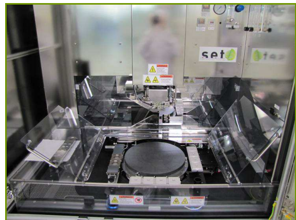
Fig. 8: Die bonder SET-FC300, modified to reach the level of particle contamination enabling direct metallic bonding
