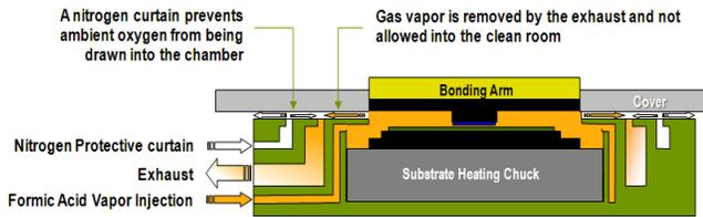
**Figure 4.** Schematic of local confinement chamber.
