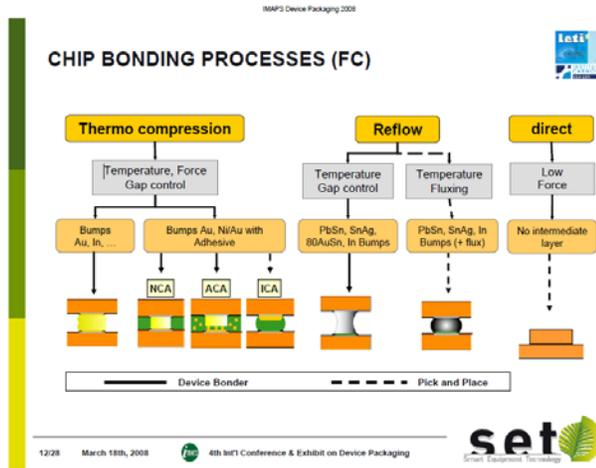
Figure 7. Matrix of chip bonding processes.
