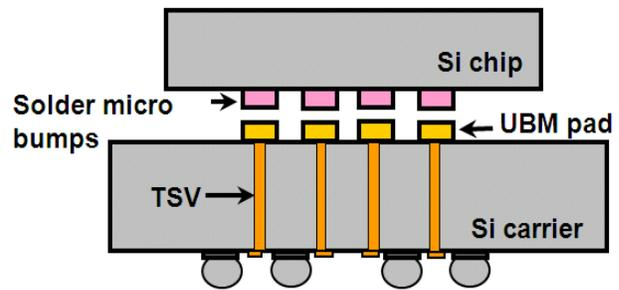
**Figure 3.** Schematic drawing of 3D stacking of the Si chip/Si carrier with TSV (not to scale). Image courtesy of A. Yu of IME Singapore.
